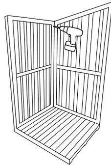
Fix the walls to the base step by step. It is advised to do this step for two people together as one can hold and the other screw. Determine screwing points yourself. Each panel needs 2 screws (50mm long) for fixing it to the floor base. **Walls need to be screwed on top of the floor base!** Start by mounting the front wall.
