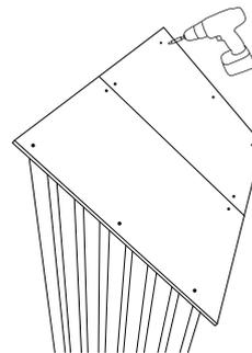
Both roof plates need to be carefully placed on the intended place for them. It is advised to do this step for two people together. Roof plates need to be screwed by 35mm screws.
